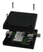
When using the **housing for 32 mm DIN- rail** the SIM- card- connector is positioned on the right side of the device.
